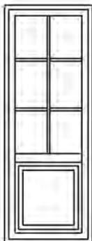
Balcony 1 door with lower boss and inglesina outside glass
